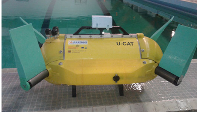
Fig. 10. View of the robot with increased floatability, a piece of float fixed to the body of the robot increases its buoyancy.
