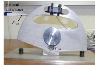
Fig. 6: Punctual disturbances applied to the pendulum
