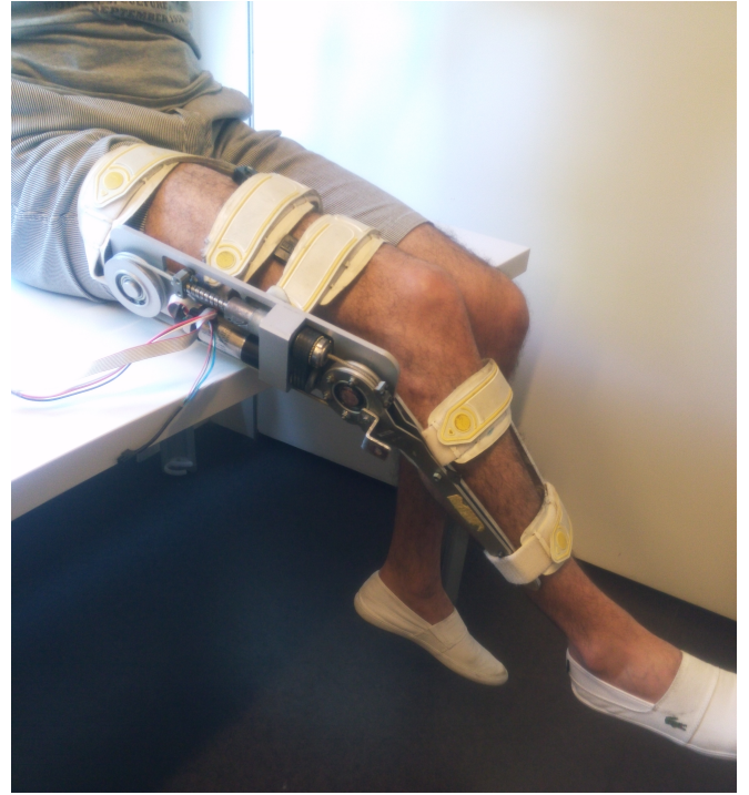
Fig. 4. The shank-foot-exoskeleton system during experiments.
