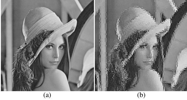
Figure 4: a) Raw image: 256 KB, b) crypto-compressed JPEG image with quality factor set to 75: 35 KB, PSNR: 20.31 dB.
