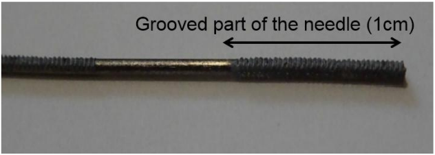
Figure 5: Schematic (a) and picture (b) of the Nitinol needle after fiber laser etching.
