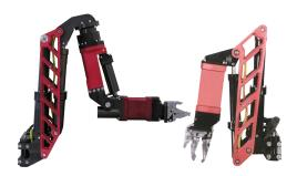
Fig. 1. Manipulator arms of Ariane: the 6-DOF (left) and 4-DOF (right).
