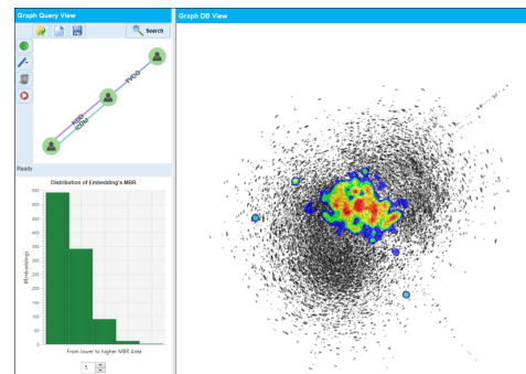
Figure 4: Visualization of the DBLP dataset. On the left, the graph query. On the right, the multilayer graph database including a Heat Map visualization showing dense areas w.r.t. the submitted query.
