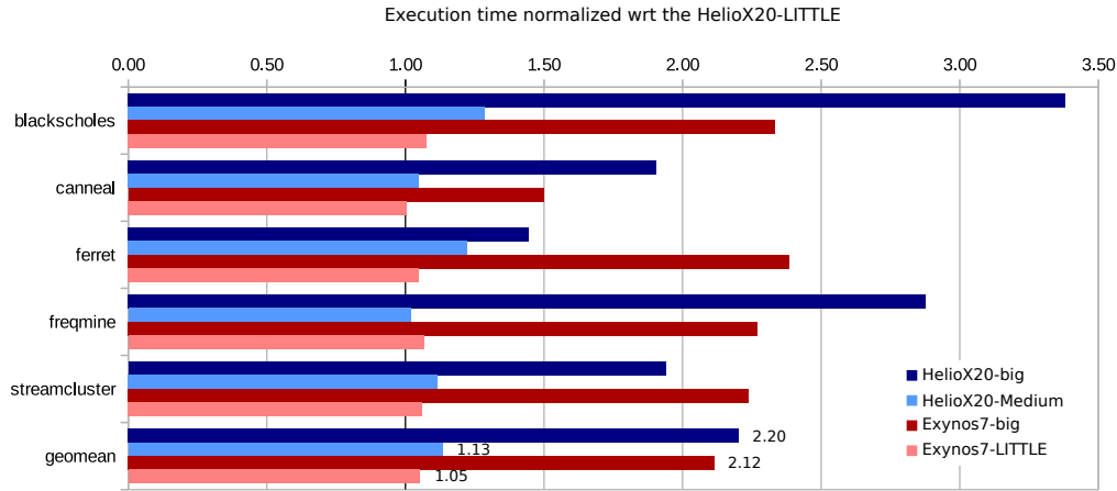
Fig. 3. Core performance relative to the HelioX20 LITTLE core. The execution times include the Region of Interest of the simlarge input set.
