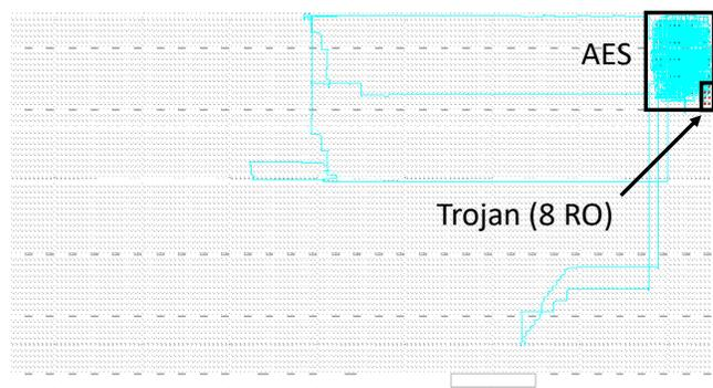
Fig. 1. FPGA layout for a stealthy Trojan insertion
