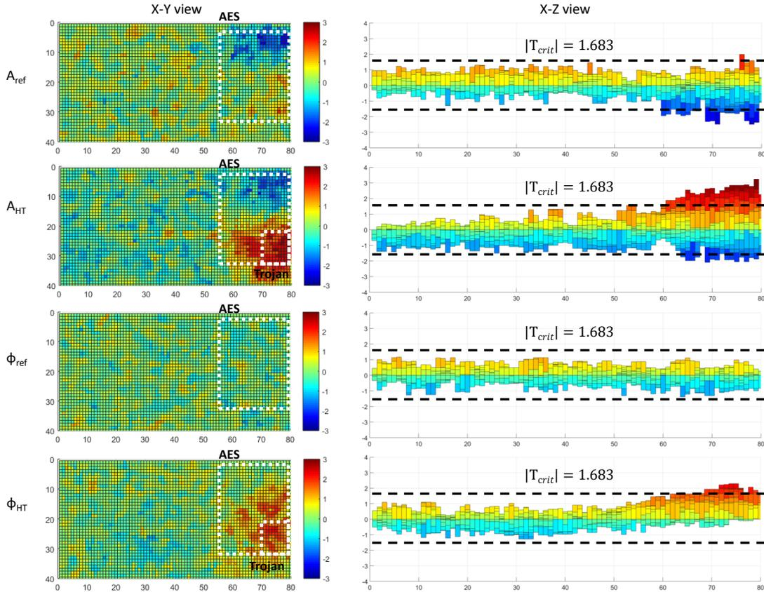
Fig. 2. Comparison between amplitude and phase results on Welch's T-test.  $A_{ref}$  and  $\Phi_{ref}$  correspond to T-values obtained by application of Welch's T-test between to golden circuits for amplitude and phase measurements.  $A_{HT}$  and  $\Phi_{HT}$  represent T-values obtained by application of Welch's T-test between a golden circuit and a HT infected circuit for amplitude and phase measurements. The dotted lines show the critical T-values (bilateral test)  $\pm T_{crit}$
