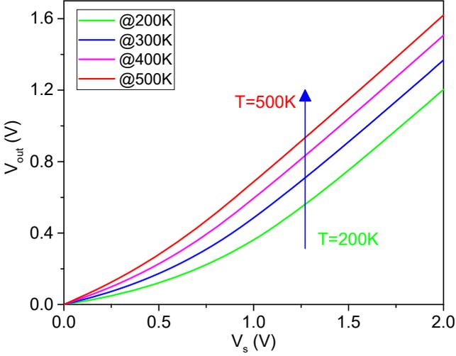
Fig. 6. The output voltages of TAC circuit under different voltage supplies and temperatures. The voltage elevates with the temperature, which is used to tune the gate voltage of  $N_{C0}$  automatically.
