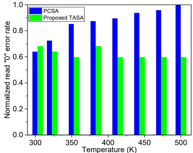
Fig. 10. Reading “0” error rates of STT-MRAM under the temperature variations. The error rates increase with PCSA, but it almost keeps constant with TASA when the temperature elevated, which has the biggest error rate reduction (almost 40%) in 500K.
