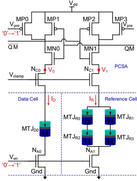
Fig. 4. The circuit of pre-charge sensing amplifier, data cell and reference cell. The resistance of the data cell branch is less than that of the reference cell. When  $V_{pre}$  and  $V_{en}$  are set to ‘1’ from ‘0’, and  $V_{clamp}$  is enabled, the discharge current  $I_D$  is larger than  $I_R$ .  $\overline{QM}$  will decline faster than  $QM$ . As  $\overline{QM}$  reaches the threshold voltage of inverter,  $\overline{QM}$  will discharge to ‘0’, and  $QM$  increases to ‘1’.
