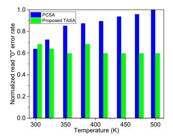
Fig. 10. Reading "0" error rates of STT-MRAM under the temperature variations. The error rates increases with PCSA, but it almost keeps constant with TASA when the temperature elevated, which has the biggest error rate reduction (almost 40%) in 500K.
