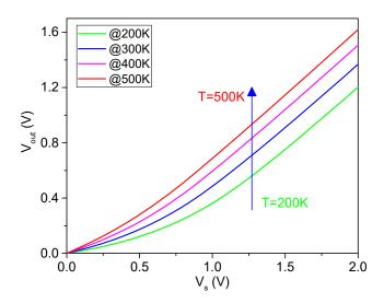
Fig. 6. The output voltages of TAC circuit under different voltage supplies and temperatures. The voltage elevates with the temperature, which is used to tune the gate voltage of  $N_{\rm C0}$  automatically.
