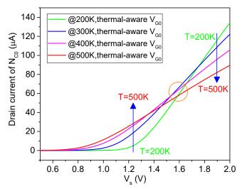
Fig. 7. The drain current of  $N_{\rm C0}$  under different  $V_s$  and the temperature variations. The drain current increases with the temperature before the brown circle, but decreases after it.
