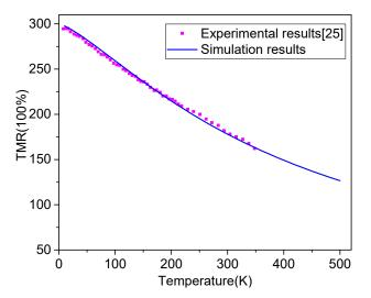
Fig. 2. TMR under the temperature variations, which is drew with (5). The magenta points are experimental results, and the blue line is the simulation results derived by the proposed model. It fits well with the experimental results in the specified temperature range.
