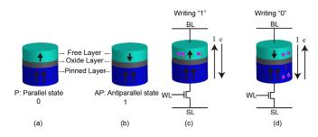
Fig. 1. The basic cell structure of STT-MRAM. (a) MTJ in parallel (low resistance) state; and (b) in antiparallel (high resistance) state, respectively; (c) writing "1" operation: from the parallel state to antiparallel state, and (d) writing "0" operation: from the antiparallel state to parallel state.
