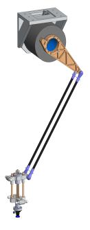
Fig. 2. Schematic view for one kinematic chain of VEIOCE robot.
