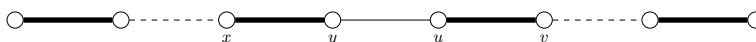
Fig. 6: Tightness of the approximation ratio. Edges are bold ( \in M^* ), solid ( \in X_{opt} ) or dashed ( \in X ) and all edges have weight one. The multiplicities of the matching edges are equal to two and the multiplicities of the non-matching edges are equal to one. Thus, \omega(X) = 2 and \omega(X_{opt}) = 1 .
