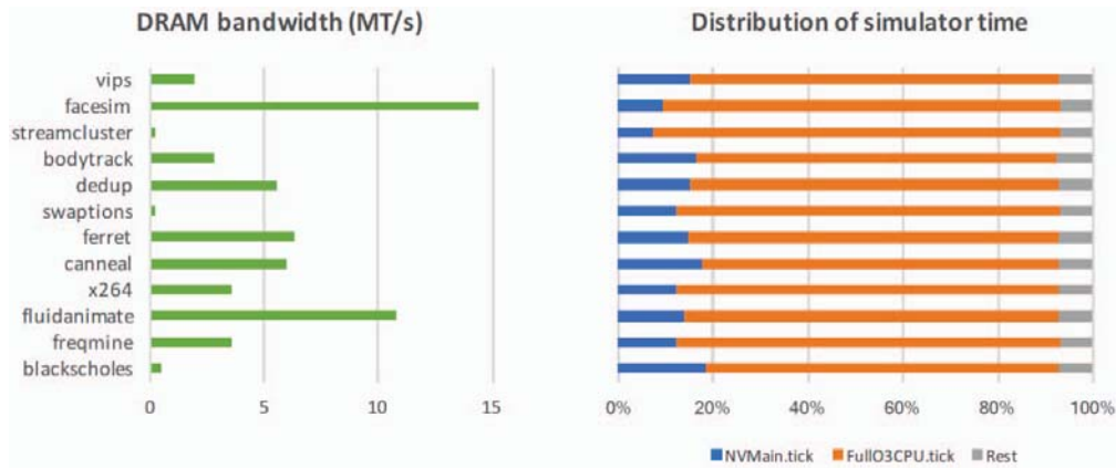
Fig. 5. DRAM bandwidth and Full System simulation time breakdown.
