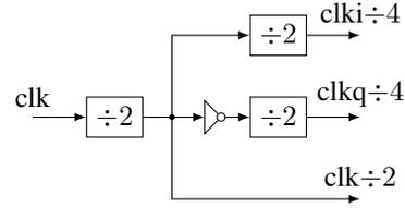
Fig. 5. Details of the "Freq. Divider" block.
