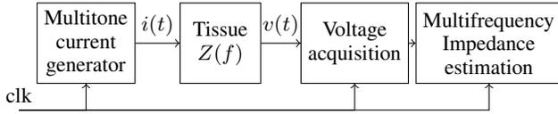
Fig. 2. Principle of multi-tone synchronous bioimpedance sensing system.
