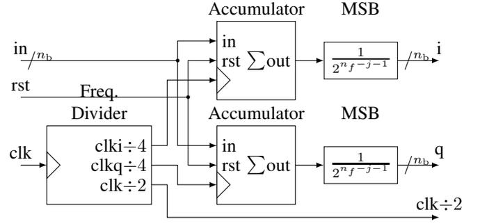
Fig. 4. Details of the "Demodulator" generic block.
