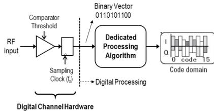
Fig.7: Industrial setup for the proposed digital technique
