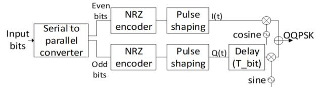
Fig.13: OQPSK modulator with half sine pulse shaping
