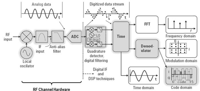
Fig.6: Current industrial setup for testing RF devices
