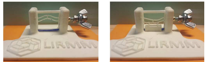
Fig. 11. Bistable curved beam (left) as shaped stable position, (right) other stable position limited by stop blocks.
