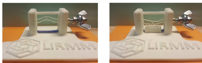
Fig. 11. Bistable curved beam (left) as shaped stable position, (right) other stable position limited by stop blocks.
