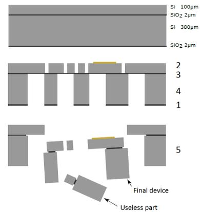
Fig. 5. Fabrication process steps.  $\text{SiO}_2$  hard mask etching on the backside (1), gold layer deposition (2), device and handle layers etched using DRIE process (3-4), structure releasing from the wafer using HF wet etching (5).
