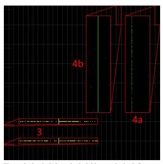
Figure 3: Logical/chronological bitmap obtained from an mMats+ test with nitrogen (LET 1.8 MeV.cm<sup>2</sup>.mg<sup>-1</sup>) on DUT #3, exhibiting SEE types 3, 4a and 4b.
