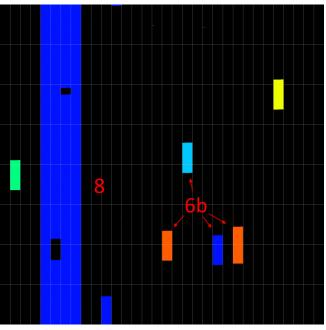
Figure 7: logical bitmap from a natural Dynamic Classic test with krypton (LET 32.1 MeV.cm<sup>2</sup>.mg<sup>-1</sup>) on DUT #2, exhibiting a type 8 and several type 6b events.
