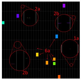
Figure 1: Logical/chronological bitmap obtained from an mMats+ test with xenon (LET 64.3 MeV.cm<sup>2</sup>.mg<sup>-1</sup>) on DUT #1, exhibiting SEE types 1a, 2a, 2b and 6a.
