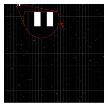
Figure 4: chronological bitmap obtained from a Dynamic Stress test with argon at 30° on DUT #4, with SEE type 5.
