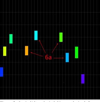
Figure 2: Logical/chronological bitmap obtained from a Dynamic Classic test with xenon (LET 60 MeV.cm<sup>2</sup>.mg<sup>-1</sup>) on DUT #1, showing SEE type 6a for comparison with Fig.1.
