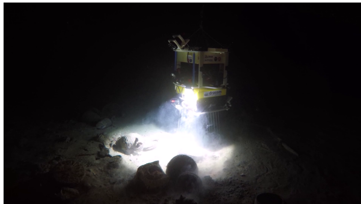
Figure 1. Remotely Operated Vehicle Dumbo performing archaeological sampling on an antic shipwreck in the Mediterranean Sea (460 m deep). This archaeological operation has been performed under the supervision of the French Department of Underwater Archaeology (DRASSM), in accordance with the UNESCO Convention on the Protection of the Underwater Cultural Heritage. Credit: F. Osada, DRASSM - Images Explorations.
