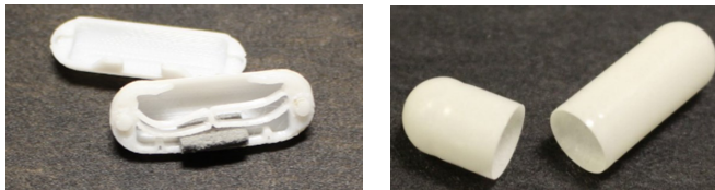
(a) Capsule assembly and integration of the dry sponge (b) Gelatin-based coating for the sampling capsule
