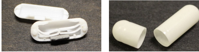
(a) Capsule assembly and integration of the dry sponge (b) Gelatin-based coating for the sampling capsule
