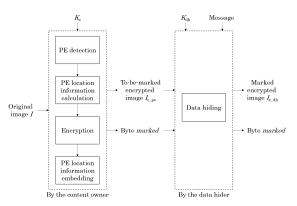
Figure 1. Overview of the encoding phase of our proposed EPE-based HC-RDHEI method.
