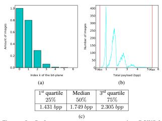
Figure 5. Performance measurements on the BOWS-2 database [1], using our proposed EPE-based HC-RDHEI method: (a) Amount of images where the data embedding phase can be achieved depending of the index k of the bit-plane (with  $0 \le k \le 6$ ), (b) Image repartition according to the payload value (in bpp), (c) Repartition by quartile of the results presented in b).
