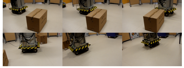
Figure 12: Snapshots of the real sensor-based navigation experiment employing the complementary route ICR controller.
