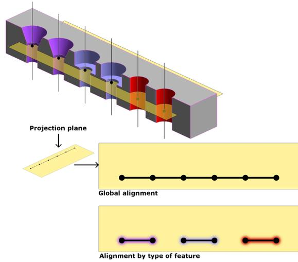
Figure 4: Axis and point alignments as 2D patterns in a reference plane.
