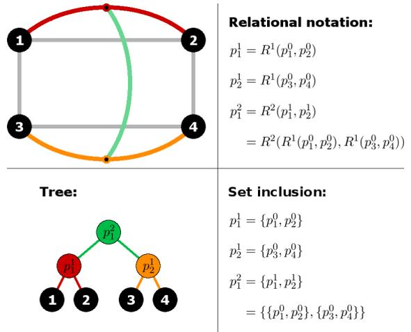
Figure 6: Equivalent notations to represent a repetition.
