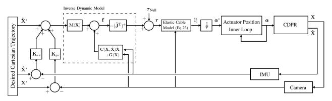
Fig. 3. Cartesian model-based control of elastic cable CDPRs, with an actuator position inner control loop.
