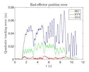
Fig. 8. Quadratic tracking error: IKC (green), KVS (blue) and DVS (red).
