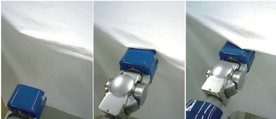
Figure 2 Participant’s field-of-view during the experiment: The participant was able to see the robot’s arm touching the curtain through the HMD, which provides visual feedback from the robot’s embedded RGB-D camera.
