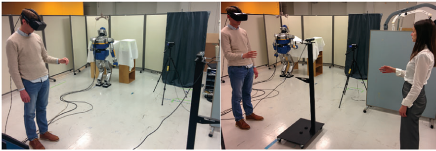
Figure 1 Setup for the synchronous (left) and asynchronous (right) conditions. The participant wears an HMD which displays visual feedback from the robot field-of-view. The participant's arm movement is tracked using the RGB-D camera (Asus XtionPRO live) and synchronized to the robot's arm movement in the synchronous condition. In the asynchronous condition, the RGB-D camera tracking the movement is turned toward the experimenter so that s/he can perform the control in place of the user.
