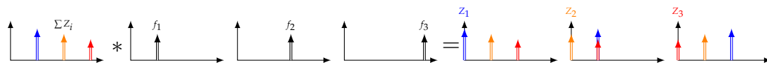
Figure 4. Conceptual representation of impedance spectroscopy based on multi-frequency excitation and Fourier analysis in frequency domain.
