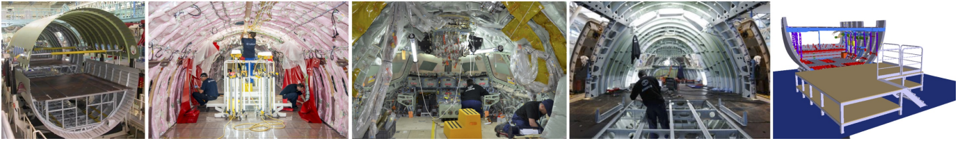
Fig. 1: Examples of the working areas and conditions in aircraft manufacturing sites. From left to right: cargo area; kneeling and using a small ladder to access the roof; cockpit area; removal of temporary floor to access in between levels; finally, CAD digital model at 1:1 scale of the A350 mockup used to demonstrate the technologies, gathering most of these scenarios.
