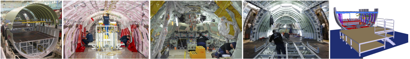
Fig. 1: Examples of the working areas and conditions in aircraft manufacturing sites. From left to right: cargo area; kneeling and using a small ladder to access the roof; cockpit area; removal of temporary floor to access in between levels; finally, CAD digital model at 1:1 scale of the A350 mockup used to demonstrate the technologies, gathering most of these scenarios.
