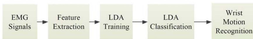
Fig. 6. Experiment process of the proposed wrist gesture classification and wrist stiffness estimation.
