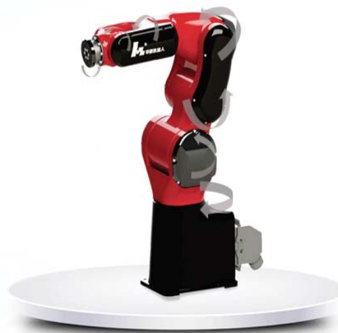
Fig. 6. The 6-DOFs robotic arm used in our system
