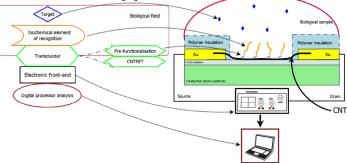
Biosensor functional decomposition and analogy to the CNTFET structure in design
