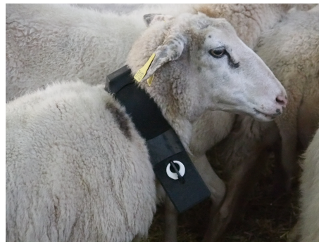
Figure 1: An accelerometer mounted on a sheep's collar.
