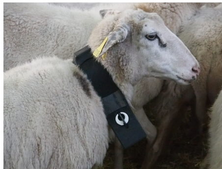
Figure 1: An accelerometer mounted on a sheep’s collar.
