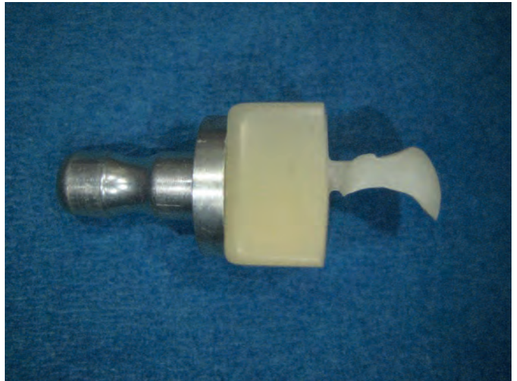
Fig.9: Crown milled in VITA ENAMIC block.
