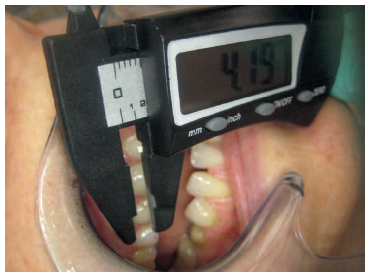
Fig.3: Digital calliper (75 mm mini digital calliper, Faithfull CALDIG 75, Faithfull) measurement for calibrating the reconstructed surface. Points are marked directly on the tooth surface with a surgical skin marker pen.
