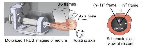
Fig. 3 TRUS probe motorization and US imaging:  $\theta$ , r and d represent the rotation increment, the rotation radius and the distance between the neighboring US frames, respectively
