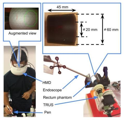
Fig. 9 Experimental setup: a surgeon marks the rectum phantom based on the augmented endoscopic view
