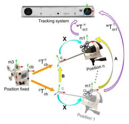
Fig. 5 hand-eye calibration to estimate transformation  $\mathbf{X}$  ( $^{m1}\widehat{\mathbf{T}}_c$ ) between the endoscopic camera c and the marker m1
