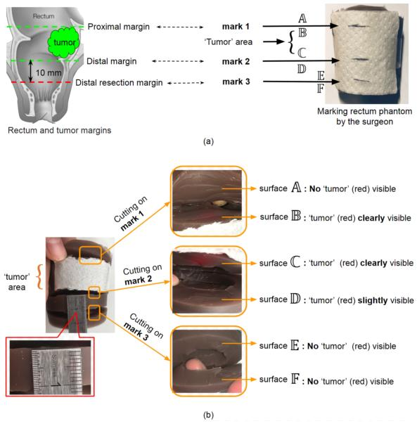
Fig. 11 Experimental results: (a) the marks (which indicates the proximal/distal margin of the tumor and the distal resection margin) on the rectum phantom; (b) cutting on the mark 1, mark 2 and mark 3 and analyzing the surfaces
