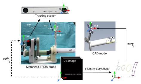
Fig. 4 US calibration process using a 3D-printed calibration phantom
