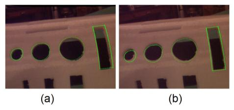
Fig. 8 Projection of the US segmentation onto the left (a) and the right (b) views of the 3D endoscopic camera
