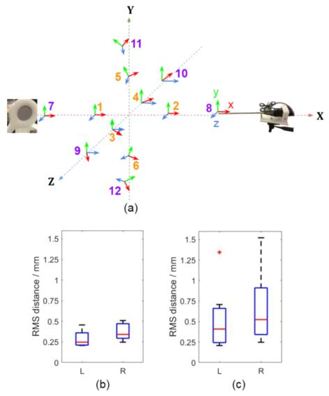
Fig. 7 (a) Endoscopic camera capturing the reflective disk in 12 poses (normal poses 1 to 6 and extreme poses 7 to 12); boxplot of  $D_{rms}$  values for the left (L) and the right (R) augmented views, when the endoscope operating in normal poses (b) and in both normal and extreme poses (c)
