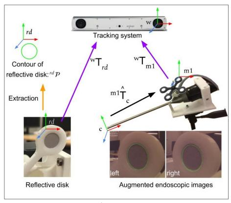
Fig. 6 Evaluating the hand-eye calibration solution  $^{m1}\widehat{\mathbf{T}}_c$  by projecting the reflective disk contour on the endoscopic images
