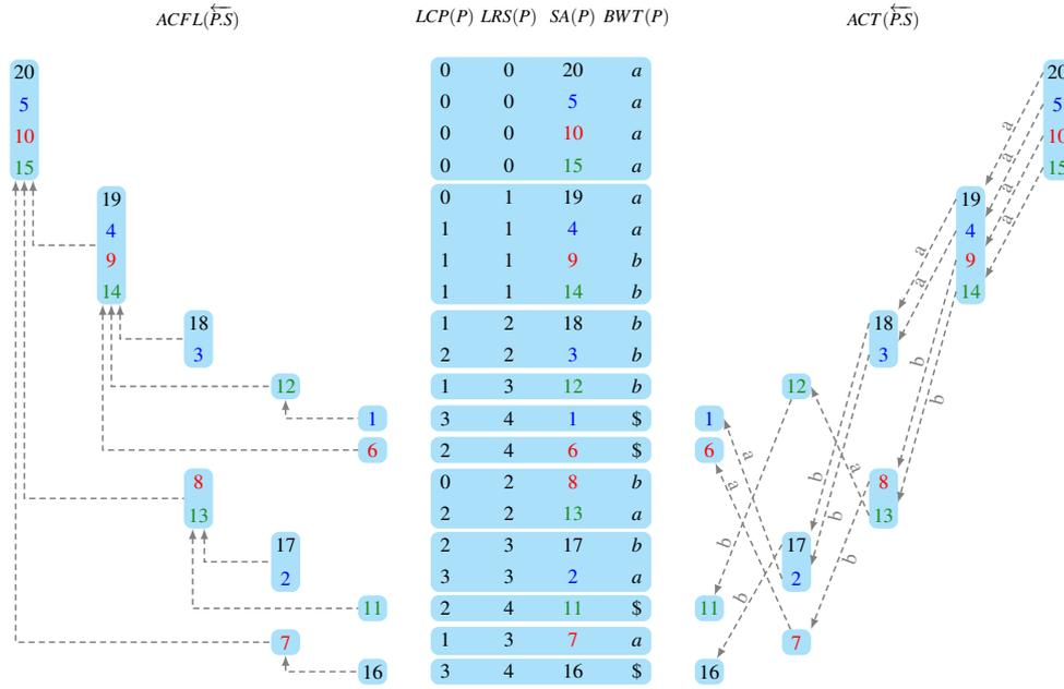
■ **Figure 4** Link between  $BWT(P)$ ,  $ACT(\overleftarrow{P.S})$  and  $ACFL(\overleftarrow{P.S})$  for the running example. The blocks in the tables SA, LCP, LRS and BWT show the decomposition  $Decomp\_BWT(P)$ .
