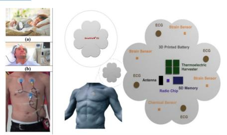
Illustration of SmartVista smart wearable device for continuous health monitoring.
