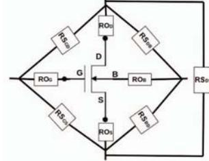
Figure 4: Considered transistor defects
