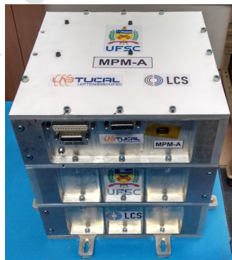
Figure 19: MPM-A instrument after acceptance tests - ready for flight
