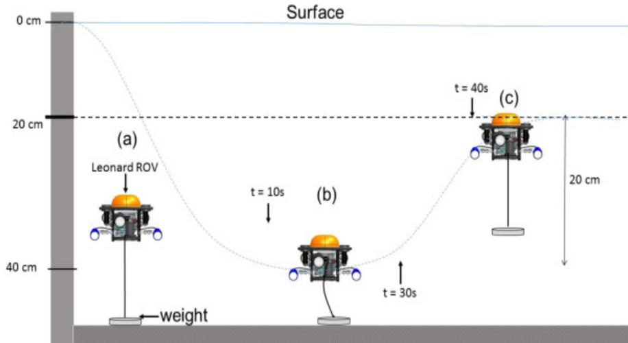
Figure 3: Description of the third scenario. (a) A  $1\text{ kg}$  load is attached to the Submarine. When the robot reaches  $30\text{ cm}$ , the influence of the weight disappears (b). Finally, the robot comes up again and the influence of the weight acts again on the robot (c).
