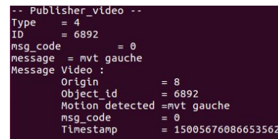
Figure 14: Terminal view from the Gateway showing the publication on the "Video" topic of a right to left motion (Mvt gauche) event
