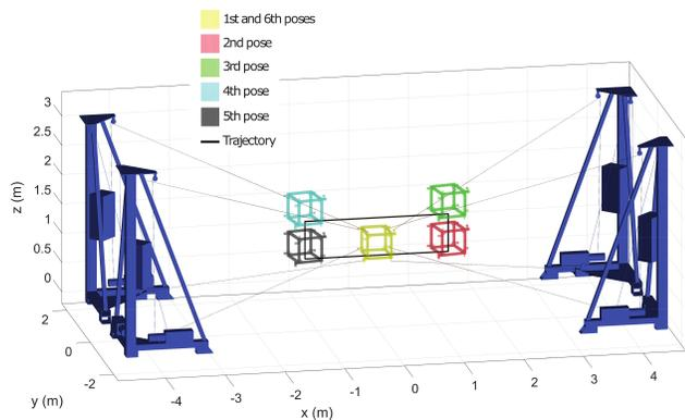
Fig. 4. Pick-and-place path and CAD view of HRPCable.
