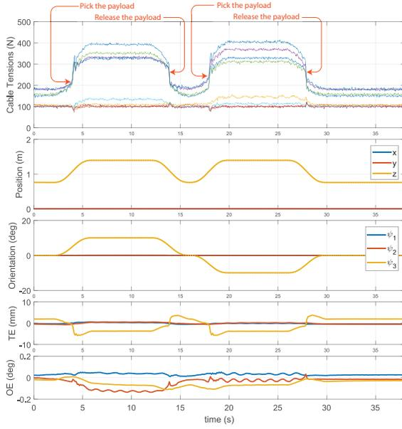
Fig. 6. Robustness test results with an additional payload.
