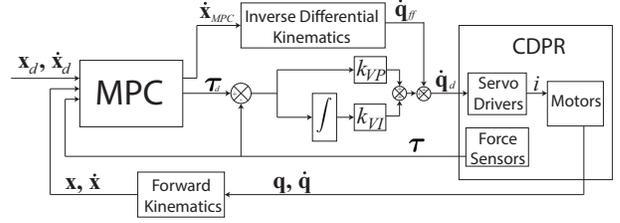
Fig. 2. Overview of the proposed control scheme
