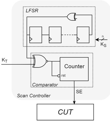
Fig. 2. Structure of the proposed scan controller.
