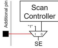
Fig. 3. Bypassing the scan controller during manufacturing test.
