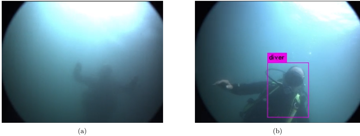
Figure 9: Underwater images from U-CAT's camera in open water conditions (a) Frame example where visual detection is not successful due to poor visibility conditions. (b) Frame example where the diver is successfully detected when close enough.
