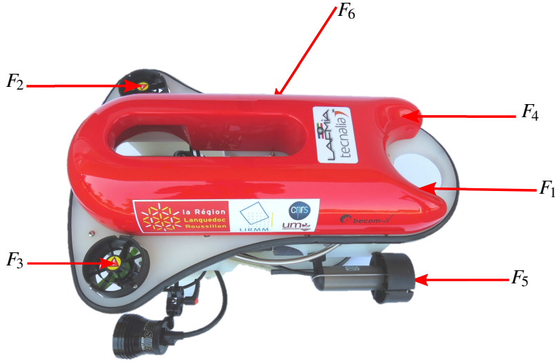
Figure 1: View of Leonard underwater vehicle thrusters' allocation, which produces forces responsible for the navigation of the vehicle.
