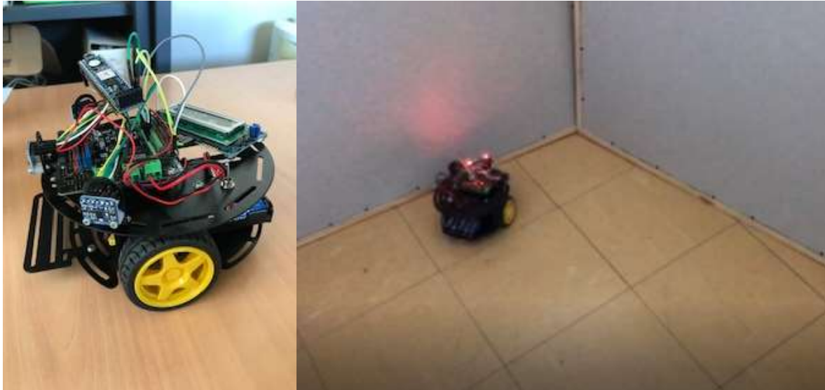
Figure 1. A mobile robot with proximity sensors controlled by ONN neural network to avoid obstacles.
